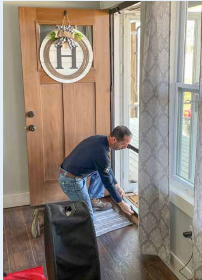
Energy Advisor Jude Canchola prepares to conduct a blower door test, a diagnostic tool that determines how much air is entering or escaping a home. Photo: Whitney Duvall
