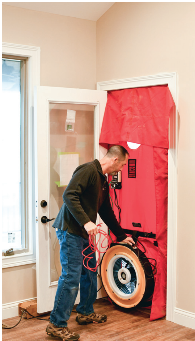
Residential Services Manager Jude Canchola performs a blower door test on a newly-constructed home built to Touchstone Energy Home standards. Photo: Whitney Duvall
